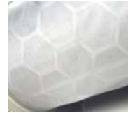
SS 316 Grade 75 Micron Mesh
